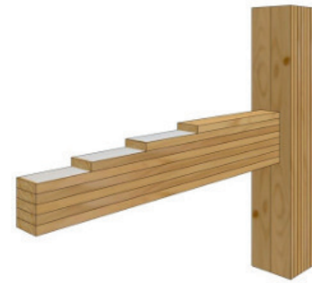
Glue-laminated timber Example Illustration from government of Canada's "State of Mass Timber", 2021
